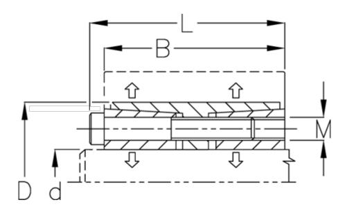
B mm = 54d H8 mm = 32D mm = 60Fit tolerance = Aksel h8, Nav H8
